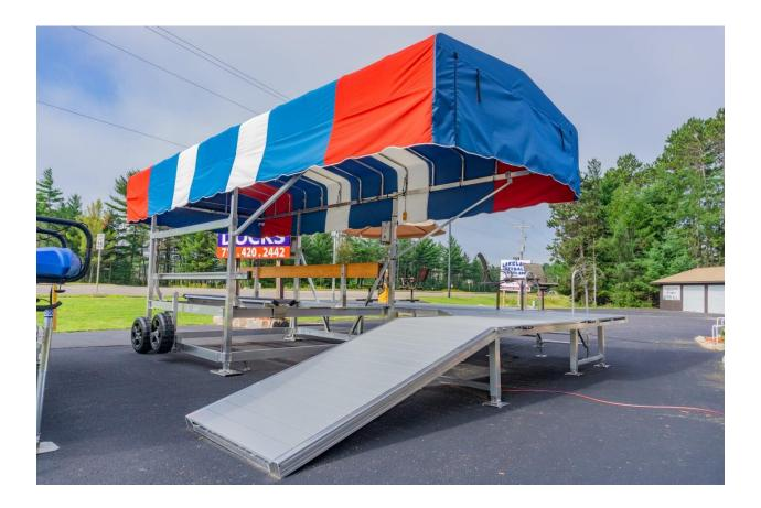
The Craftlander Canopy System consists of the canopy legs, canopy frame, canopy fabric and the canopy fabric attachment system. The canopy fabric attachment system is made up of bungees for the sides and for the ends of the fabric.
