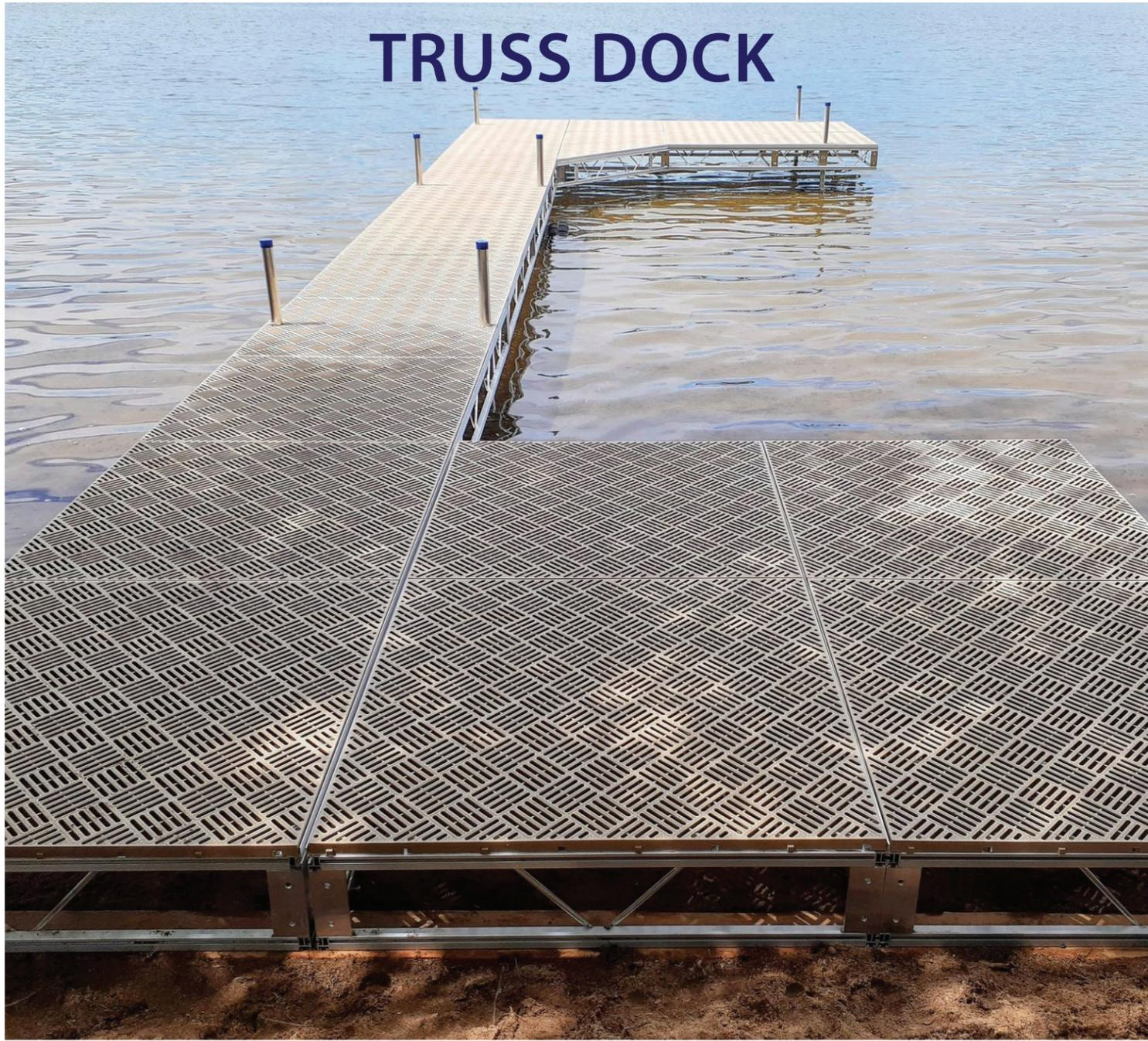
Truss Docks boast a lightweight classic design, and provides the ultimate ease going in and coming out of the water. Sturdy aluminum trusses with cross members every 12" means your dock won't shift or flex. Truss Docks can be installed with wheels or legs, depending on your shoreline. Removable 4'x4' decking panels allow you to match your dock to your needs and environment.
